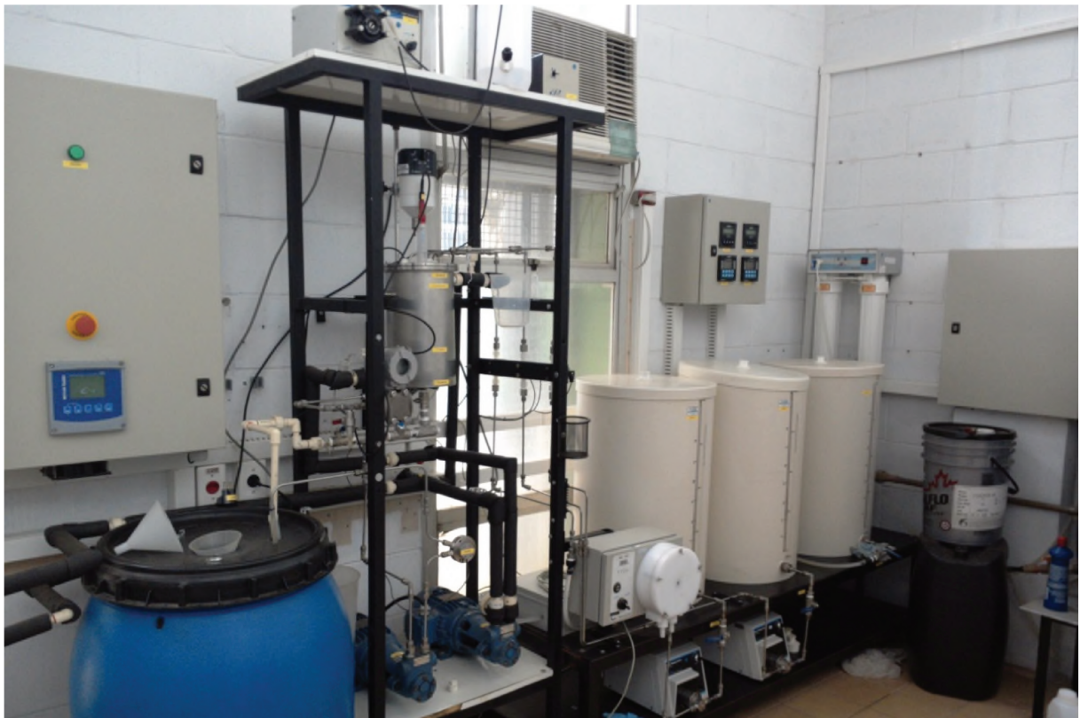
Figure 15 – Experimental plant for the neutralization reaction. (LCAP/FEQ/Unicamp)
