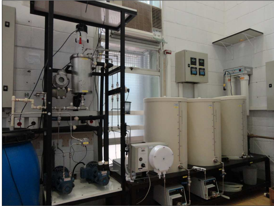
Figure 21 – The experimental pH neutralization plant.
