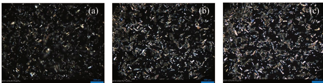
Fig. S4 Images captured using an optical microscope of 1 wt% cellulose in 2-HEAPr. (a) T = 30.0 °C; (b) T = 69.7 °C; (c) T = 100.0 °C
