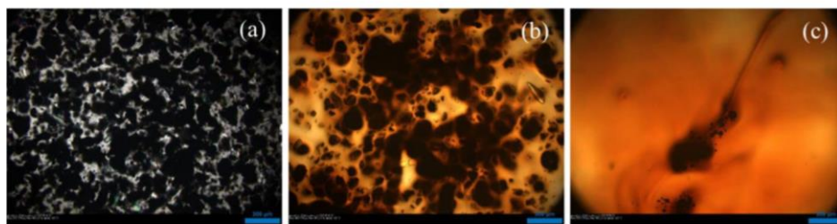
Fig. 10 Images obtained by optical microscope of lignin + xylose in 2-HEAF. 5 wt% of lignin and 5 wt% of xylose in 2-HEAF at heating rate of 1.0\text{ }^{\circ}\text{C min}^{-1} : a T=30.0\text{ }^{\circ}\text{C} ; b T=44.9\text{ }^{\circ}\text{C} ; c T=57.8\text{ }^{\circ}\text{C}
