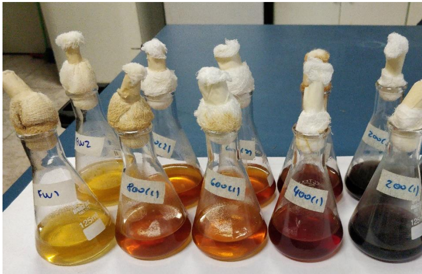
Fig. IV.4. From left to right: full wash, 800, 600, 400 and 200 wt% hydrolysates before yeast inoculation (wash at 25°C).
