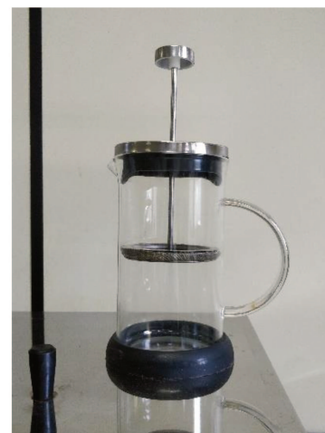
Fig. IV.1. (a) Wash water from the washing experiments (b) French press employed for solid:liquid separation of the pulp from the wash water.
