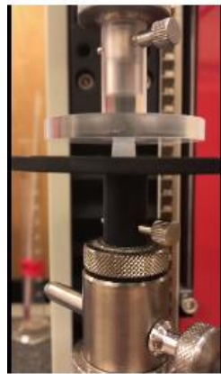
Video S1. Crosslinked 20% PEG-2.5% alginate hydrogel under a compressive strain of 30% and returning to its original shape.
