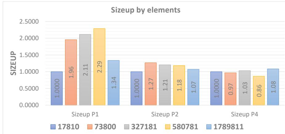
**Figure 6.46.** Sizeup by elements using the crankshaft meshes with 17810, 73800, 327181, 580781 and 1789811 elements with polynomial orders 1, 2, 4 and 6; 20 compute nodes with 1 rank MPI per node, 20 cores per node and 2 threads per core, totalizing 40 threads OpenMP.
