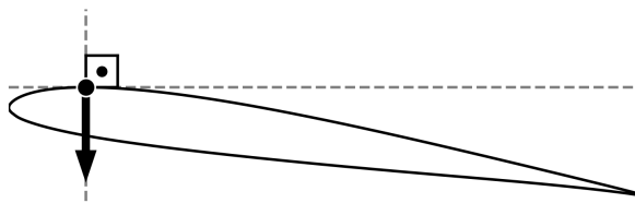
Figure 4.6: Position x_{vsn} where the inward pointing surface normal at the suction side is vertical.
